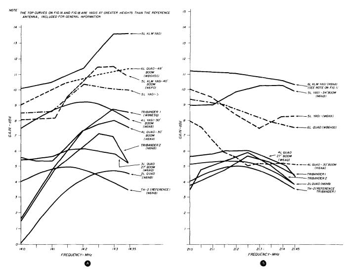
fig. 1. Relative gain measurements for 20, 15, and 10 meters. (A) shows 20 meters, (B) 15 meters, and (C) 10 meters. The top curves on 20 and 15 meters are for a Yagi which is at a greater height than the reference antenna. They were included only for general information, not for direct comparison.
